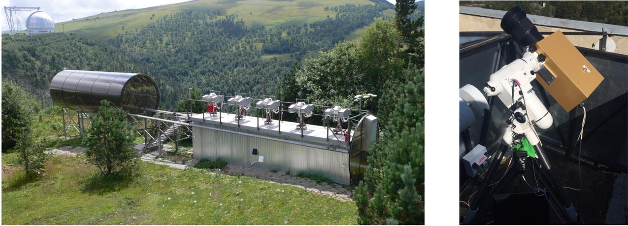
Fig. 2. The hardware used for a two-station meteor observations. Left – Mini-MegaTORTORA multi-channel system, located near Russian 6-m telescope of Special Astrophysical Observatory. Right – reconstructed FAVOR camera, located on the roof of main building of Special Astrophysical Observatory, at 3.8 km distance from Mini-MegaTORTORA.
