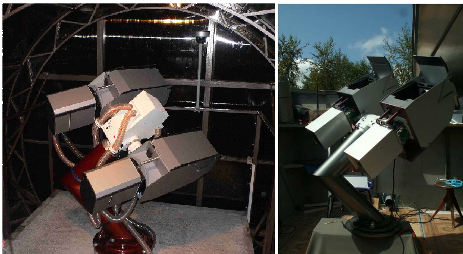
Fig. 2. Two MMT channels installed on a single mount. The complete system consists of five such mounts, carrying nine operative channels and one replacement channel.
