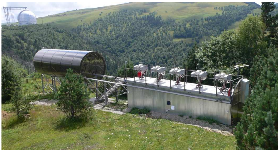
Fig. 3. All the nine MMT channels installed on five mounts in a single cylindrical dome, shown here open. The Russian 6 m telescope is seen in the background.
