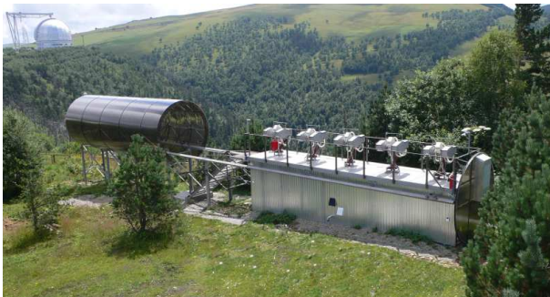
Fig. 2. Photo of the all 9 channels of MMT installed on 5 mounts in the single cylindrical dome, which is open at that moment. Russian 6-m telescope may be seen in the background.
